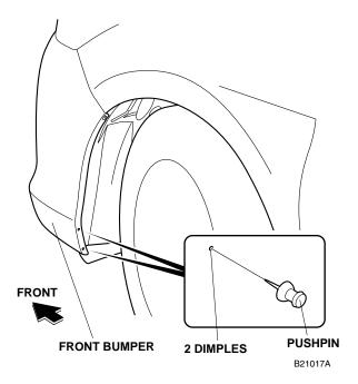
Thread a self-tapping screw into each pierced mark to make a hole in the front bumper. Remove the selftapping screw.
