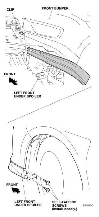
12. Check that the clip on the left front under spoiler is fully pushed into the slot on front bumper, then secure the front portion of the under spoiler to the front bumper with one washer and one bumper clip supplied.
