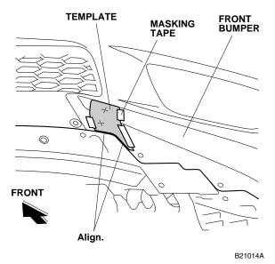
3. Using a pushpin, pierce the front bumper through the two holes in the template. Remove the template.
