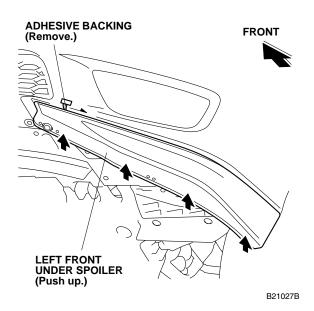
15. Using your hand, firmly press the left front under spoiler against the front bumper for 30 seconds.
