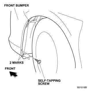
8. Install one spring nut over each hole in the front bumper in the direction shown.
