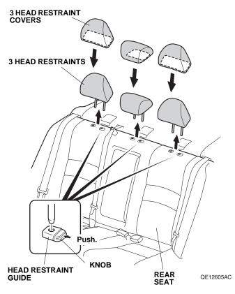
Fit the three head restraint covers over the head restraint.
