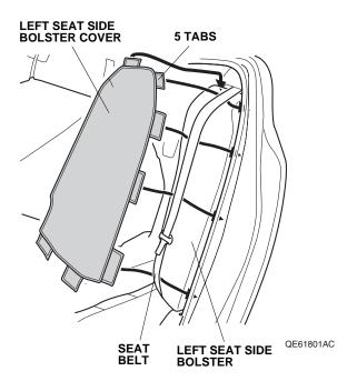
Secure the three fasteners to the left seat side bolster.
