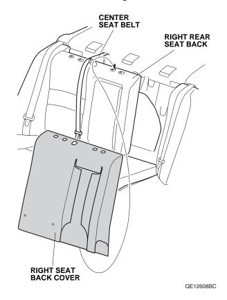
Secure the fastener on the right rear seat back.
