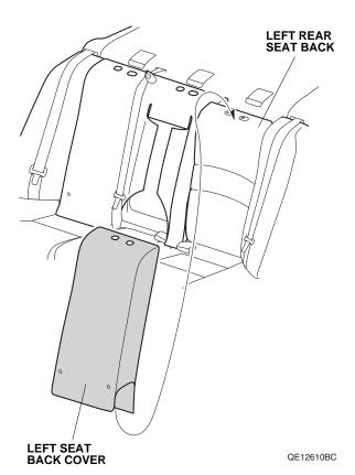
Secure the fastener on the left rear seat back. Raise the left rear seat back and lock it to its original position.
