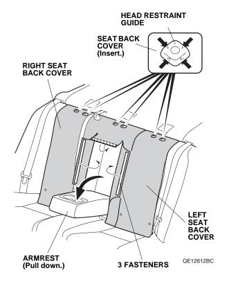
14. Insert the seat back covers between the rear seat backs and the rear seat cushion, and secure the three fasteners to the rear seat backs.
