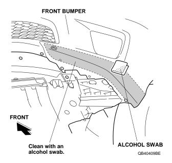
Install the left front under spoiler to the front bumper, and loosely install two self-tapping screws into the spring nuts in the fenderwell.
