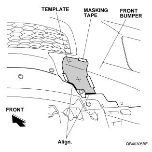
3. Using a pushpin, pierce the front bumper through the two holes in template. Remove the template.
