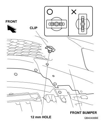
6. Using a pushpin, pierce the left front bumper at the two dimples on the front fenderwell.
