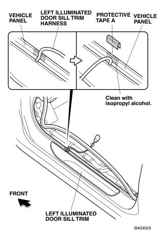
22. Install the protective clip to the protective tape A on the vehicle panel.
