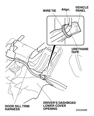
44. Secure the door sill trim harness to the vehicle harness with one wire tie. Move the steering wheel up and down through its full adjustment range and make sure the door sill trim harness is not being stretched.
