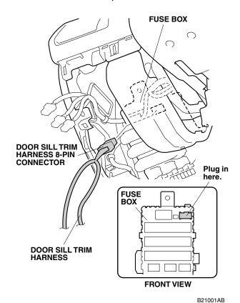
28. Remove and discard the dummy connector from the other accessory harness. Plug the door sill trim 8-pin connector into the other accessory harness 8-pin connector.
