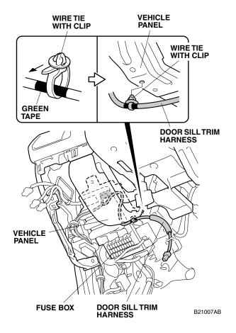
Using diagonal cutters, cut the clip portion off of one wire tie.
