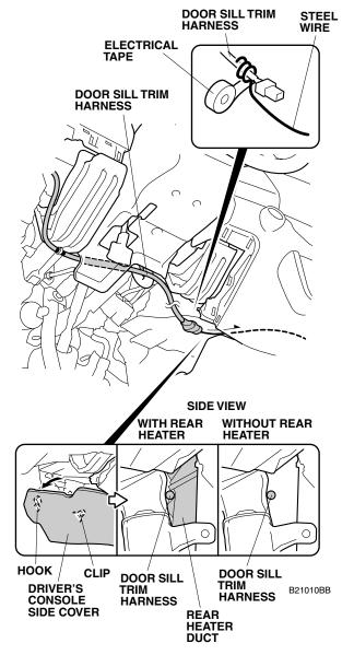
40. Attach a piece of steel wire to the door sill trim harness with electrical tape. Route the door sill trim harness through the center console from the driver's dashboard lower cover opening to the passenger's under cover opening.
