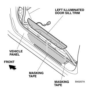
18. While applying light pressure against the left illuminated door sill trim, carefully remove the adhesive backings.
