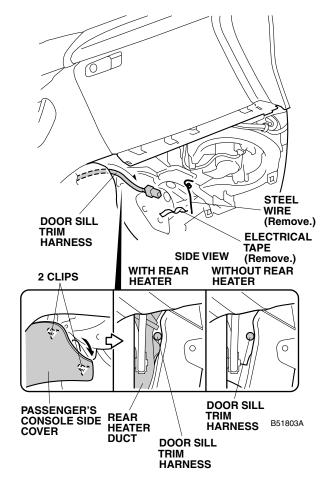
42. Route the door sill trim harness, and remove the electrical tape and steel wire.
