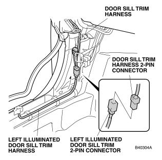
31. Plug the left illuminated door sill trim harness 2-pin connector into the door sill trim harness 2-pin connector.
