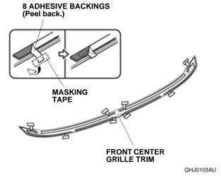
3. Line up the front center grille trim with the front grille, and attach it as shown.
