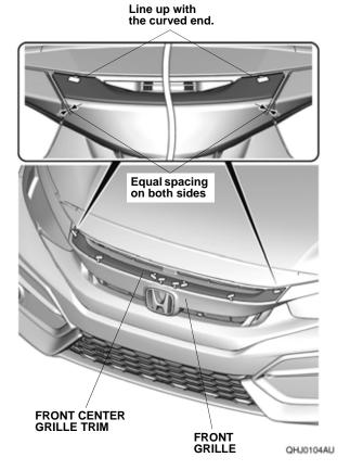
4. While applying light pressure against the front center grille trim, carefully remove the taped adhesive backings.
