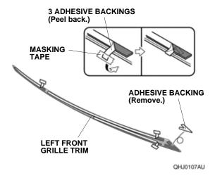
7. Line up the left front grille trim with the left front grille extension, and attach it as shown.
