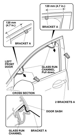
3. Install two brackets A between the door sash and the glass run channel at the measurements shown. Seat the glass run channel properly around the brackets.
