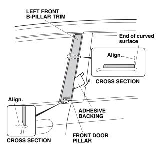
3. Using the rubber roller, apply pressure to set the adhesive.
