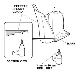
16. Install the left rear splash guard using the one self-tapping screw that you removed and two clips. Be sure not to create a gap between the left rear splash guard and the body.
