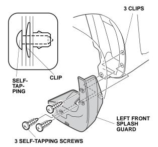
Check that the left front splash guard fits the contour of the vehicle.
