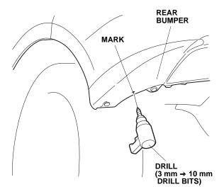
14. While wearing eye protection, drill a 10 mm hole through the rear bumper at the pierced mark. First drill with a 3 mm drill bit, then finish with a 10 mm drill bit. Remove all burrs.
