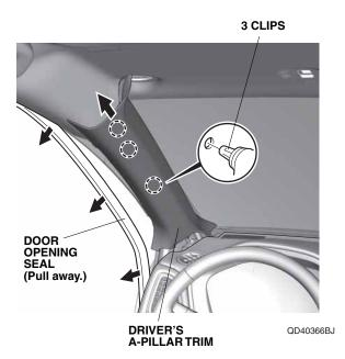
12. Pull away the door opening seal, and remove the driver's dashboard side lid.
