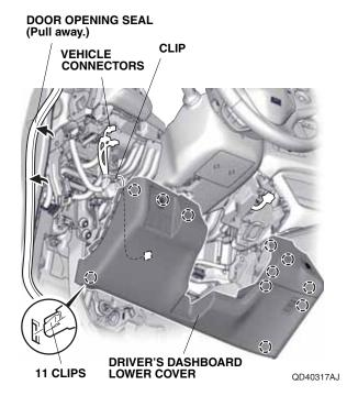
15. Pull away the door opening seal, and remove the driver's front door sill trim.
