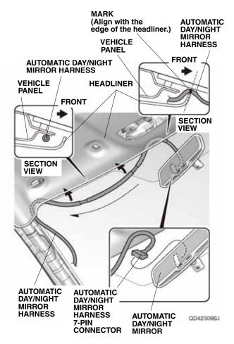
24. Gentry pull back the headliner, and tuck the automatic day/night mirror harness behind the headliner. Align the mark on the automatic day/night mirror harness with the edge of the headliner. Be careful not to crease the headliner. 25. Route the automatic day/night mirror harness through the groove in the harness cover. Secure the harness cover to the mirror stay. Slide the harness cover behind the headliner.
