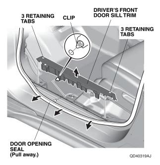
16. Pull away the door opening seal, and remove the driver's kick panel.
