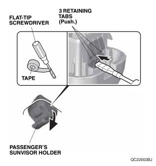
While holding down the passenger's sunvisor holder as shown, use a flat-tip screwdriver wrapped with a tape to remove the passenger's sunvisor holder.
