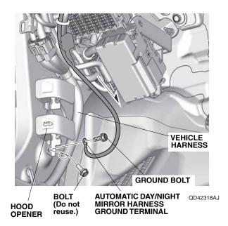
35. Secure the automatic day/night mirror harness to the vehicle harness with two wire ties.
