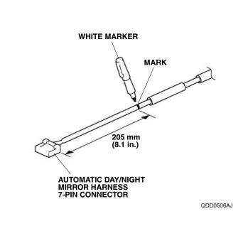
23. Plug the automatic day/night mirror harness 7-pin connector into the automatic day/night mirror.
