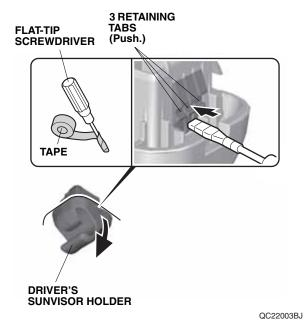
While holding down the driver's sunvisor holder as shown, use a flat-tip screwdriver wrapped with a tape to remove the driver's sunvisor holder.
