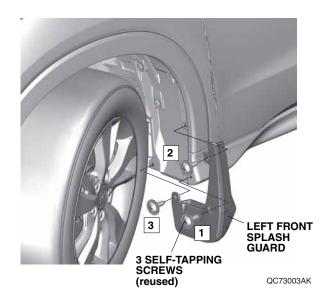
4. Remove the two self-tapping screws.
