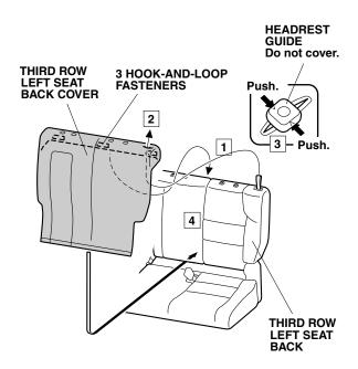
5. Fold down the third row left seat. Secure the third row left seat back cover to the third row left seat back with one hook-and-loop fastener. Return the third row left seat to the upright position.
