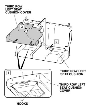
7. Secure the third row left seat cushion cover to the third row left seat cushion with the two hook-and-loop fasteners.
