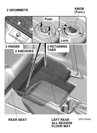
Place the grommets in the right rear all-season floor mat over the anchors. Push the grommets into the anchors to secure the retaining tabs, then turn the knobs 90° to secure the right rear all-season floor mat.
