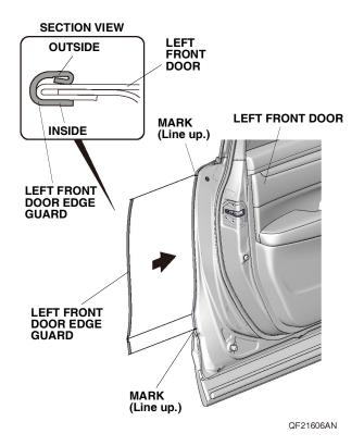
14. Starting at the feature line, use a rubber mallet to tap the left front door edge guard into position with a series of light taps, then work up and down. Make sure the position of the left front door edge guard is correct.
