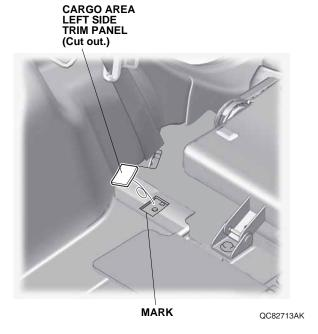
5. Install one tie-down using the bolt supplied. Torque the bolt to 9.8 N·m (7.2 lb·ft).
