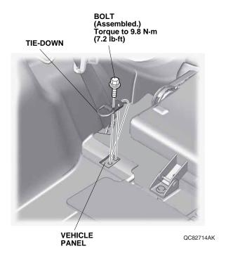
6. Repeat steps 2 through 5 to install a tie-down on the right side of the vehicle. Return the cargo board to the original position.
