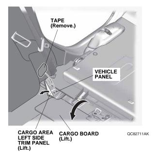
3. Put the cargo area left side trim panel down. Mark the cargo area left side trim panel at the measurements shown.
