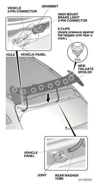
15. Connect the rear washer tube to the joint. Install the new tailgate spoiler to the tailgate with nine clips. NOTE: To confirm clip engagement, listen for a click sound during installation.
