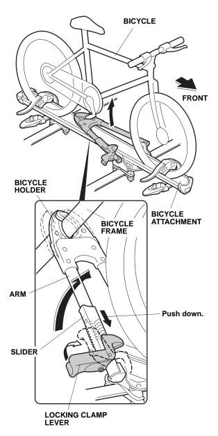
14. Push up the locking clamp lever to secure the bicycle frame.
