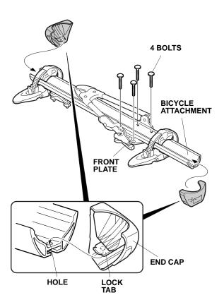
7. Install the bicycle attachment to the cross bar with two knobs, two washers, and one bracket. Repeat the same procedure for the other two positions on the bicycle attachment.
