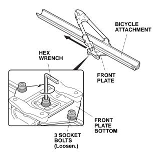
Set the front plate 245 mm (9.6 in.) from the end of the bicycle attachment as shown, and retighten the three socket bolts at the bottom. Torque the three socket bolts to 8 N·m (5.9 lbf·ft). Rotate the arm as shown.
