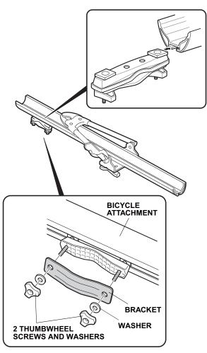
4. Slide the rear plate onto the bicycle attachment.
